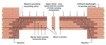
The upper tendon combines with the two surrounding brick courses to enhance compression and the bottom tendon acts in tension to significantly increase the tensile and flexural capacity of the masonry.
